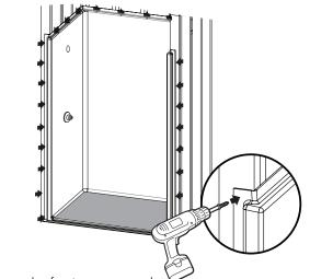
Fasten panel to framing at every stud and eight inches vertically through nailing flange.
