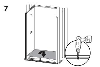
Cover the entire bottom of the unit with a piece of cardboard or other protective material. Pre-drill pilot holes and fasten unit to floor starting in the center of the base flange moving outward every 8 inches.
