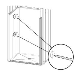
If mounting fittings — from stable reference points (back wall studs, floor) measure the locations of spout and valves. Note measurements.
