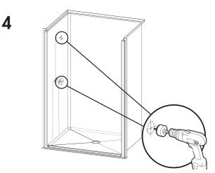
Mark fitting locations. (Refer to measurements from step 3.) Using a hole saw (fine tooth or abrasive grit cutting edge), make necessary openings for filler and valves, drilling from inside (smooth side) out.
