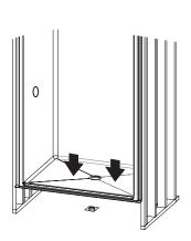
Place the unit directly on level floor (or on top of foundation materials) with drain fitting over and onto waste pipe with threshold firmly on the floor. Assure waste pipe protrudes well into drain fitting. Maintain proper floor slope towards drain.
