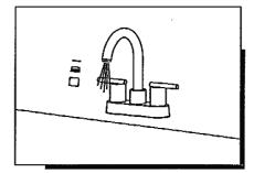
6. After installing faucet, remove aerator assembly and open the hot and cold water supplies. Check for leaks. Turn on faucet handle
