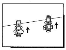
3. Re-assemble the mounting hardware, screw and tighten lock nuts onto faucet.
