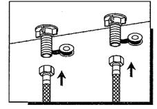
4. Apply pipe tape to threads. Attach braied hoses one end to the faucet and screw onto inlet ports.
