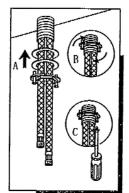
3. From underneath the sink, replace the washers and lock nut.Use philips screwdriver for final tightening after spout is aligned.
