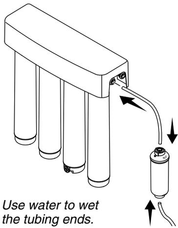
Use water to wet the tubing ends.
