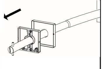
Insert screws through first mounting plate into anchors. Tighten screws until you feel increased resistance.
