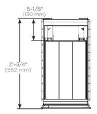
Top view for plumbing and sink clearance
