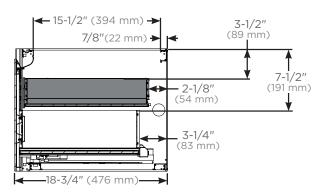
Side views for plumbing and sink clearance with door front
