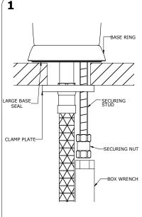
Mimas - Lever should be on the right when viewed from the front of the fitting. Hole centre a minimum of 2. 1/2" from the wall.
