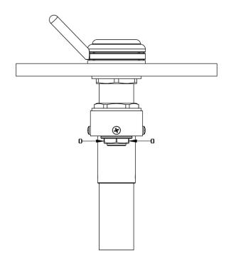
7. Tighten gear box bottom lock nut set screws. One or both set screws may be tightened.
