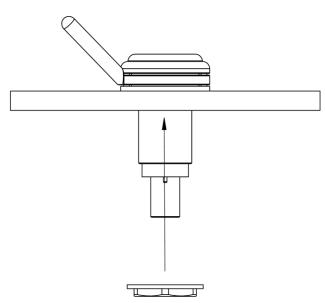
2. Tighten base onto counter making sure base is aligned so lever can turn equally to the right and to the left. Turn lever to leftmost position.
