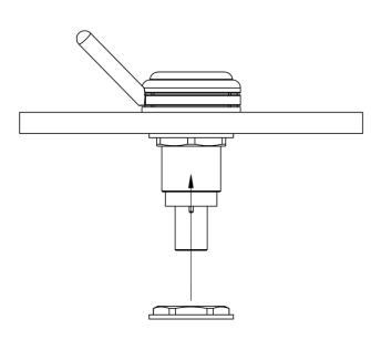
3. Screw gear box top lock nut onto base. Do not tighten.
