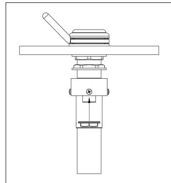
Screw gear box bottom lock nut onto base until it contacts the bottom of the gear box. Do not tighten.
